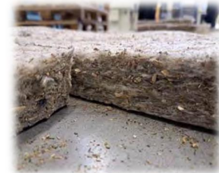
Insulation panel made with green waste
