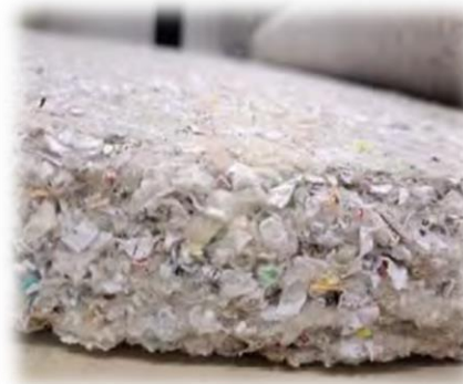
Insulation panel made with paper waste
