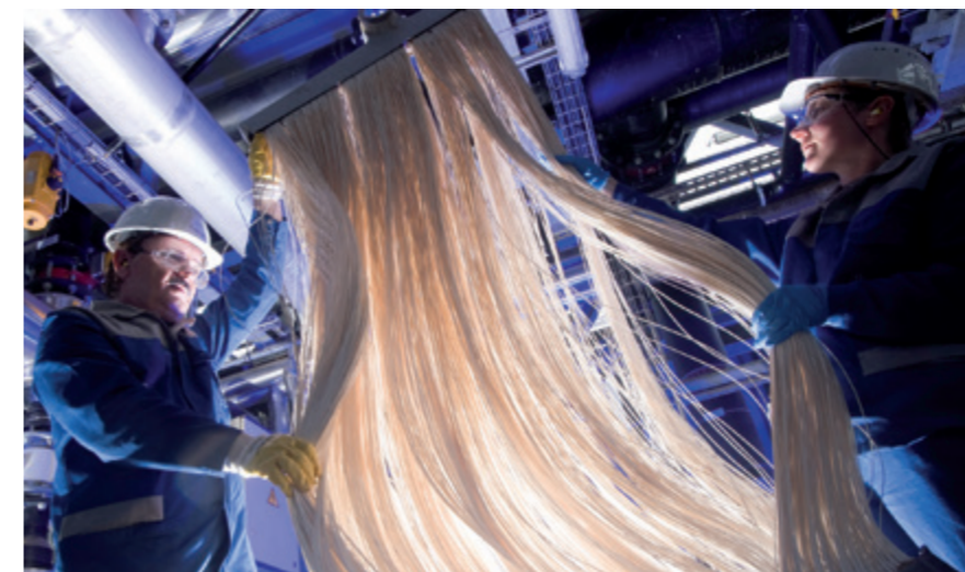
Hollow fiber membranes in industrial wastewater treatment (© Bayer Pharma AG)
