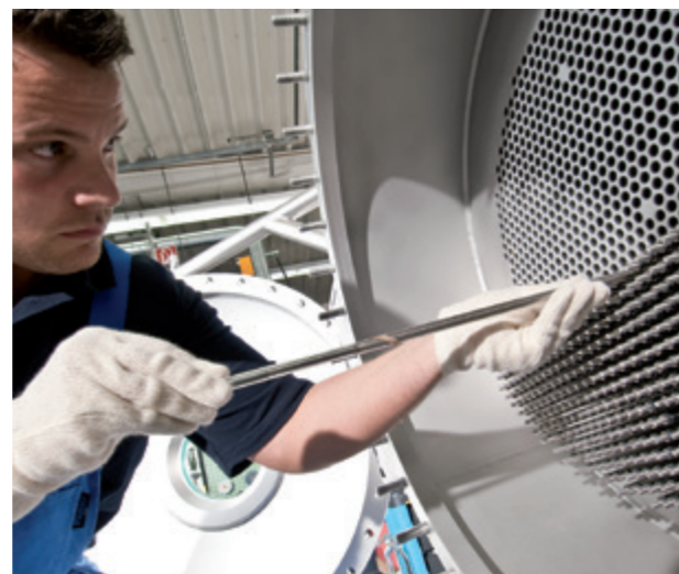
Implementation of ozone electrodes (© Xylem Inc.)
